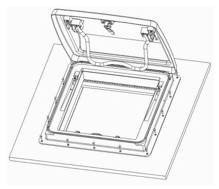
Remove the upper of the skylight, place the component into the mounting hole(outside the wall) with the opening in the direction of the rear of the caravan, use seal glue, fix with 16 pcs self-tapping screws(PA-4.8\*32).
