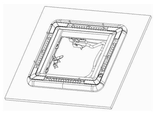
Remove the window cover, please the lower part of the skylight into the mounting hole(inside the wall) with the light switch in the opposite of the window opening, use 8 pcs self-tapping screws (PA-4\*25), put the cover.
