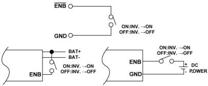
Figure 2.2.2.2 - Wiring configurations for Remote Control Green Terminal
