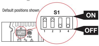
Figure 2.1.3.1 - Dip Switch ON/OFF Positions
