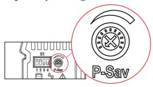
Figure 2.1.4.1 - Power Saving Load Adjustment
