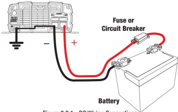
Figure 3.3.1 - DC Wiring Connections
