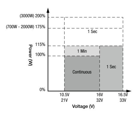
700W - 3000W Figure 1.3.1 - Input Voltage vs. Output Power
