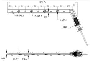
Figure 19 Dimension of PMWS400 (Unit: mm)
