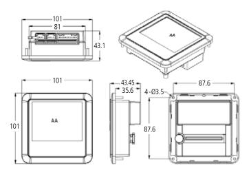
Figure 13 Dimension of Monitor (Unit: mm)
