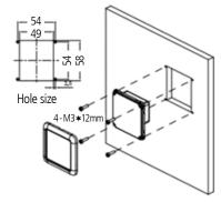
Figure 18 Installation of PM4SW2 (Unit: mm)
