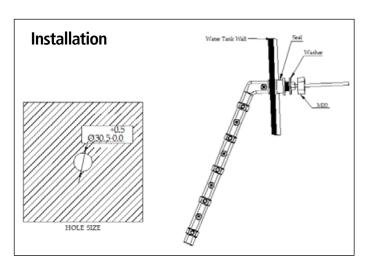
Figure 20 Installation of PMWS400 (Unit: mm)
