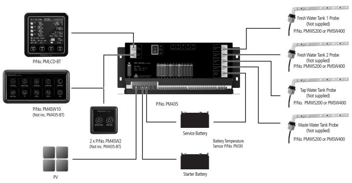
Figure 1 System Components for PM400 & PM435-BT
