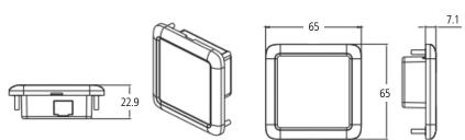
Figure 16 Dimension of PM4SW2 (Unit: mm)
