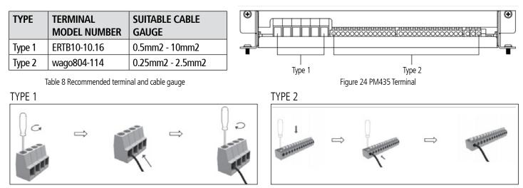
Figure 25 Connection of Terminal Type 1
