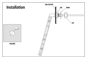
Figure 22 Installation of PMWS200 (Unit: mm)
