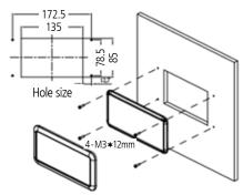
Figure 17 Installation of PM4SW10 (Unit: mm)
