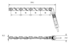
Figure 21 Dimension of PMWS200 (Unit: mm)
