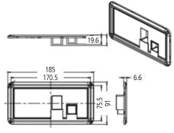
Figure 15 Dimension of PM4SW10 (Unit: mm)
