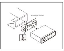
Insert mounting sleeve into the wall panel and bend the mounting tabs out with a screwdriver. Make sure that the lock lever (Fig 1) is flush with the mounting sleeve (not projecting outward)
