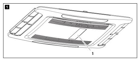
The control panel (1) is at the air outlet unit of the roof air conditioner.
