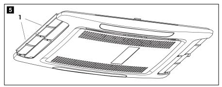
Turn the slats (1) in the air nozzles independently in the required directions. The air flow can be adjusted along the ceiling or towards the floor.
