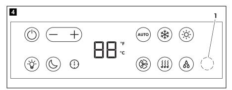
The remote control **must** be pointed at the IR receiver (1) on the control panel during operation.
