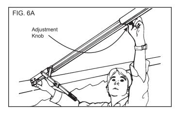
B. Grasping the tension mechanism lever, carefully move it up even with the tension rafter and slide the lock over the lever to secure the rafter. (FIG. 6B)This step pushes the roller tube out and stretches the fabric taut. The tension rafter is designed to use the full stroke of the tension mechanism for 25 foot awnings. Shorter awnings may require less tension.
