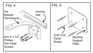
**NOTE:** Be sure to use a dab of silicone sealant on every screw or rivet where a hole has been drilled in the side of the vehicle. This will prevent possible water leakage.
