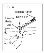
Slide lock tension mechanism up and pull lever down while holding dowel pin at end of rafter in roller tube. (FIGS. 5A & 5B)
