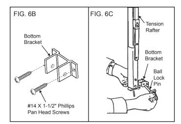
**NOTE:** When installing the tension rafter on a curved vehicle which does not allow for rafter storage, bottom bracket installation is not required.
