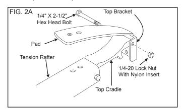
B. With awning closed, position the tension rafter at the center of the awning so that it has a minimum of 69" of unobstructed clearance below the awning rail. If windows and/or service accesses interfere, relocate tension rafter as close to center of awning as the situation will allow. (See FIG. 2B).
