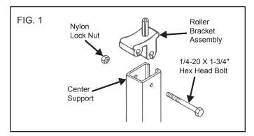
**NOTE:** If the Optima Center Support is being used in conjunction with the Optima Tension Rafter, the roller bracket is not required and the center support should be attached to the tension rafter as pictured in FIG. 2. To attach center support, use 1/4-20 nut and 1/4-20 x 2-1/2" hex head bolt in the tension rafter. Install the center support with the two rubber sleeves (provided) on both sides of the center support. (FIG. 2)
