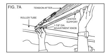
B. Slide the knob toward the vehicle and carefully swing the center support down placing the foot of the center support on the ground. (FIGS. 7B, 7C & 7D)
