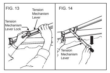
15. Loosen adjustment knob on side of tension rafter and push tension mechanism lock up, slide tension mechanism lever down. (FIGS. 14A, 14B & 14C)
