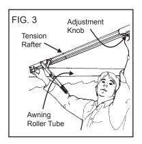
4. Extend tension rafter and attach it to awning roller tube by inserting dowel at end of rafter into drilled hole in roller tube. (FIG. 4)
