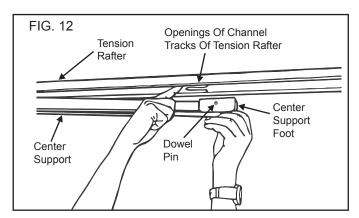
Make sure the pin is seated inside the channel tracks of the tension rafter before securely tightening the larger 1-7/8" adjustment knob.
