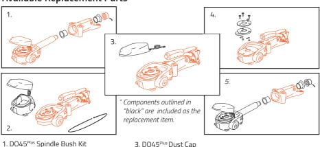
1. DO45<sup>Plus</sup> Spindle Bush Kit (18D-DO45-SPINDLE-BUSH-PLUS)
