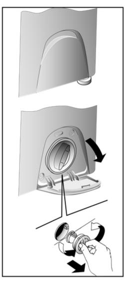
Attention: if the filter needs cleaning while there is washing still in the drum, follow the instructions on the following page to empty the water. This will prevent excessive loss of water via the filter.
